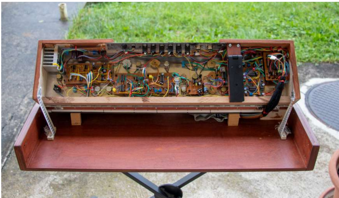
Picture 6.2 This picture shows all electronics. Also, the heatsink on the top left and the stand on the right is visible. The ribbons on both sides stop the upper part from overrotating and destroying the hinge.
