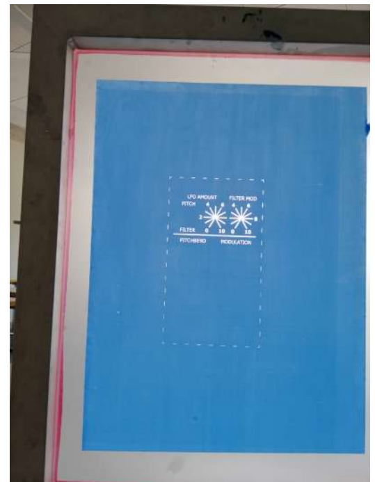
Picture 3.5 The finished screen is ready for printing the labels for the wheels-panel.
